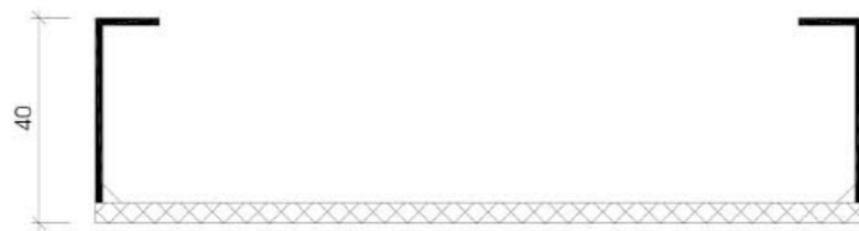
明框 Version 3 : Welded-on Frame
