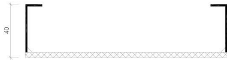
隐形框 Version 1 : Welded-on Frame
