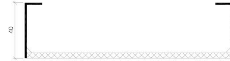
浮框 Version 4 : End-welded tp expanded metal
