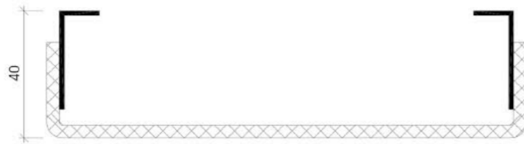
隐形框 Version 2 : Bend with inside welded frame
